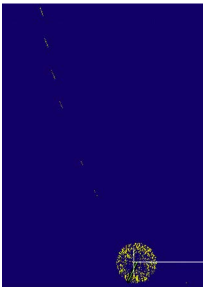
Figure 114 Typical interference from another radar
