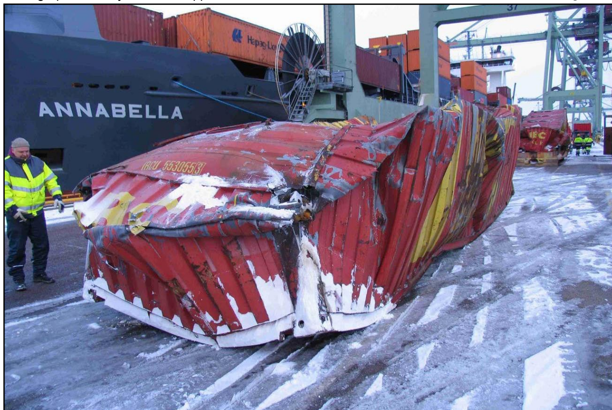
Lowest container discharged at Kotka, 5 March 2007
