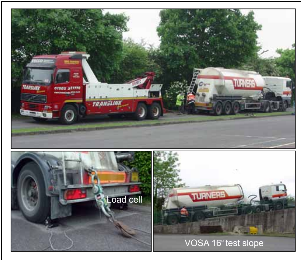
Wheel chock performance tests
