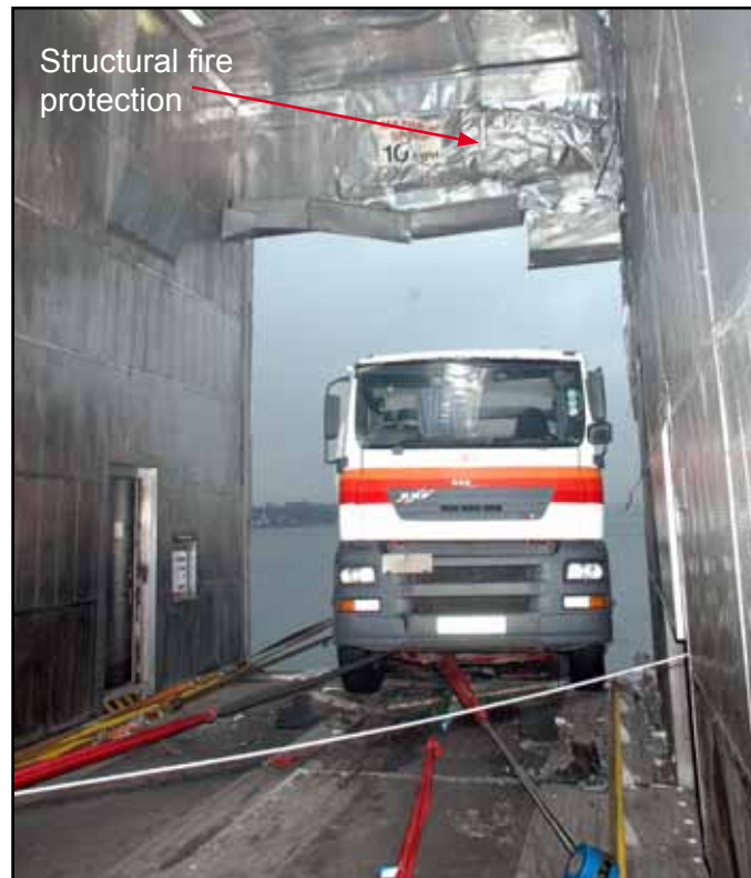
Road tanker tractor unit secured to the deck
