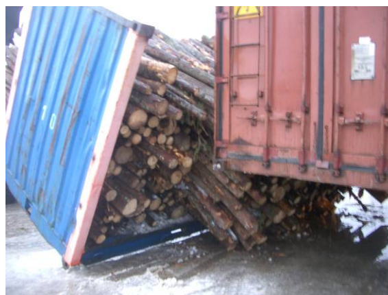
The logs started to move against the painted steel sheet at 30°.
