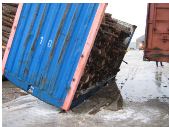
A container, handled by a fork lift, was used to prevent the logs from moving too far away from the container flat.
