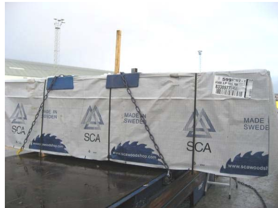
Pictures illustrating the assembly of chains used for producing the pulling force.
