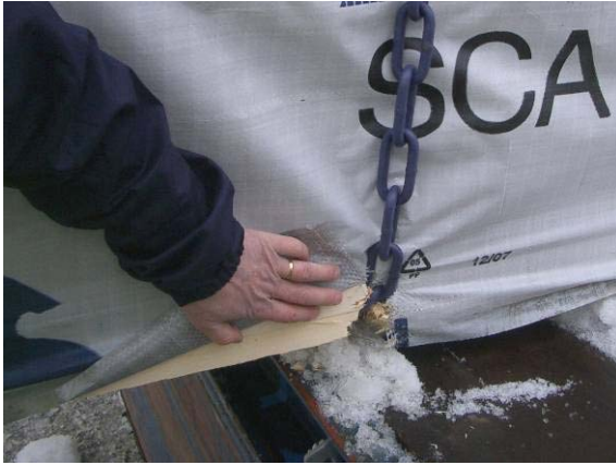
Chain cutting through timber
