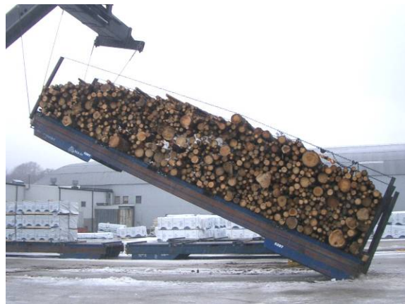
20° inclination. The logs have shifted towards the lower end.
