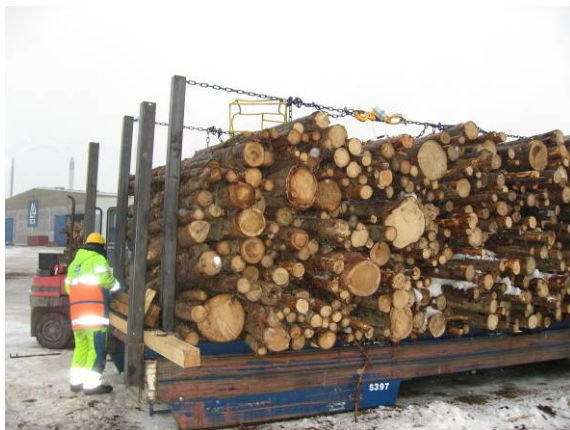
Loose uprights supporting the logs at one end of the flat. The uprights were bottom blocked and supported by chains at the top.
