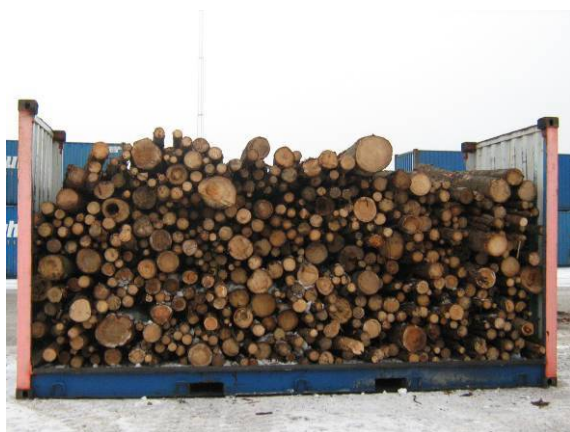
20' Container flat with fixed gables loaded with approximately 20 ton pulp wood.
