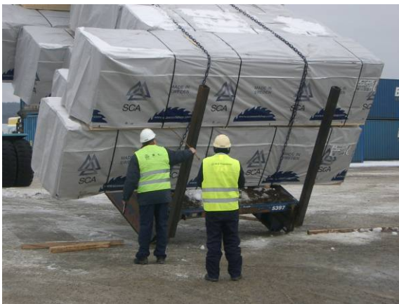
Measuring of distances to the uprights at the lower end.
