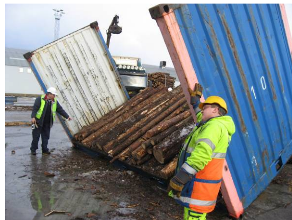
The logs on plywood slid at 32°.
