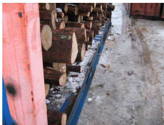
All logs in the bottom layer were stowed at least 10 cm from the angle bar along one of the sides of the flat
