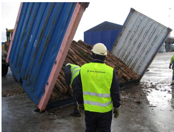
The logs on steel sheets slid at 21°.
