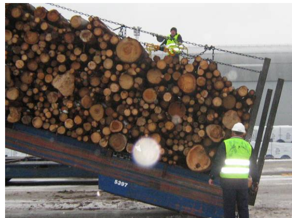
Forces in the chains were measured with dynamometers.
