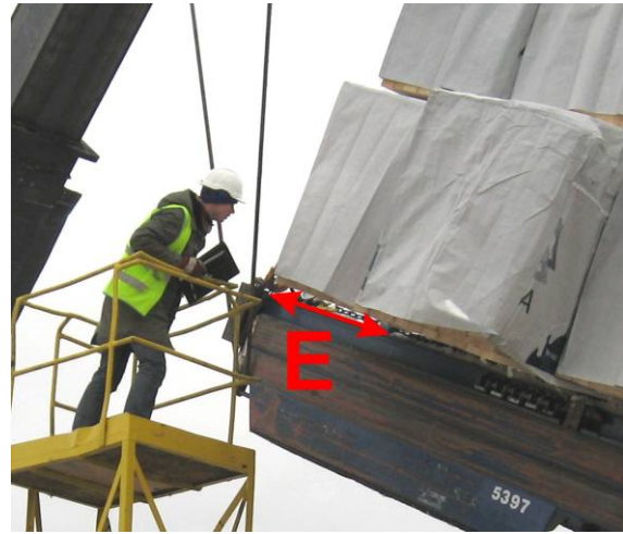
Distance between the cargo and the end of the platform at the high end.
