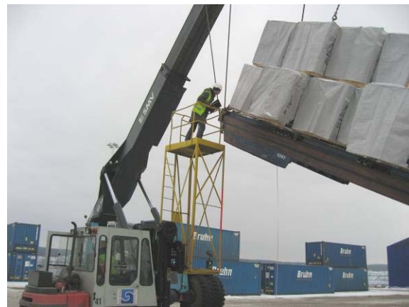
Measuring of distance and lashing forces at the high end.
