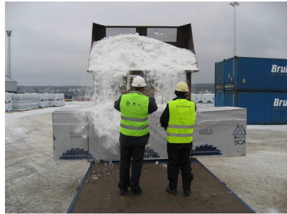
Snow being sprinkled on top of the bottom package to obtained winter conditions.
