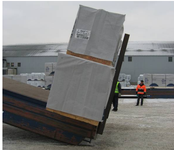
Inclination test with two packages. The upper package is free to slide while the bottom one is blocked against the uprights.
