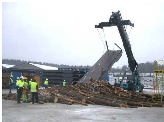
After collapse at 34° inclination
