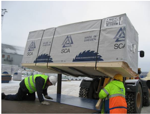
Painted steel sheet used underneath the cargo to simulate the material contact between timber and the deck of a vessel.
