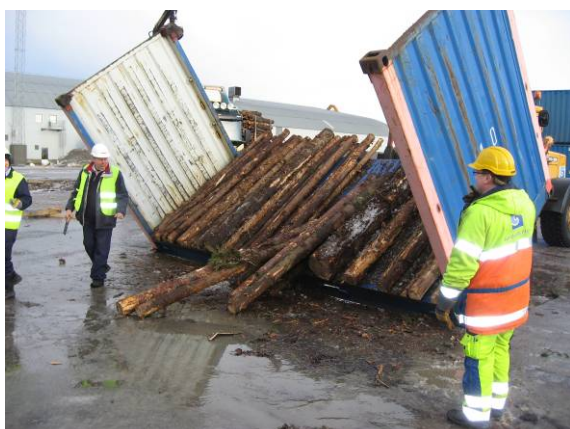
The logs in the top layer slid at 38°.
