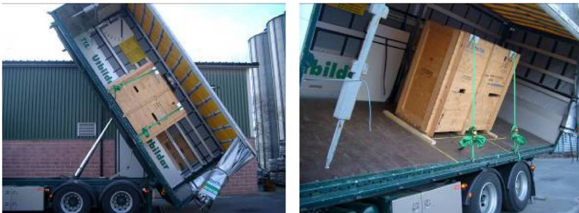
The cargo securing arrangement of a heat exchanger is tested for acceleration forces forward and sideways.
