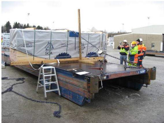
Pictures illustrating the assembly of chains used for producing the pulling force.
