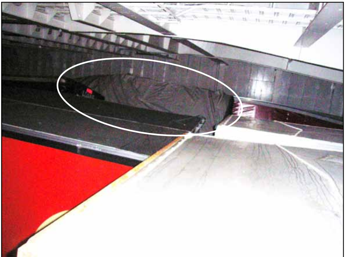
Trailers still secured on the main deck after grounding - note the flatbed with load still secured (circled)
