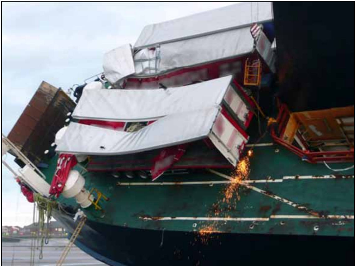
Aft deck - trailers remain secured at large angle of heel
