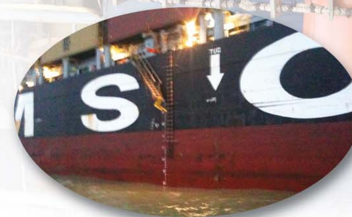
Ladders can injure vessel crews too! An A.B. on this vessel fell into the North Sea in October 2010 when this accommodation ladder platform collapsed under him. The man, wearing just a boiler suit with no life jacket or PPE, was retrieved by the Pilot Cutter. He was treated by Paramedics and returned to his ship, unscathed. The cause of the accident, according to the Master, was a failed weld, on a repair made a few weeks earlier.
