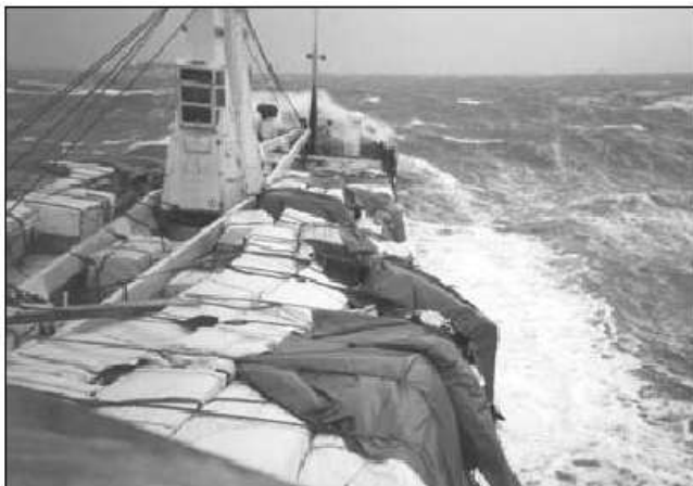
Fig. 3 Shifting cargo on a ship in a storm
