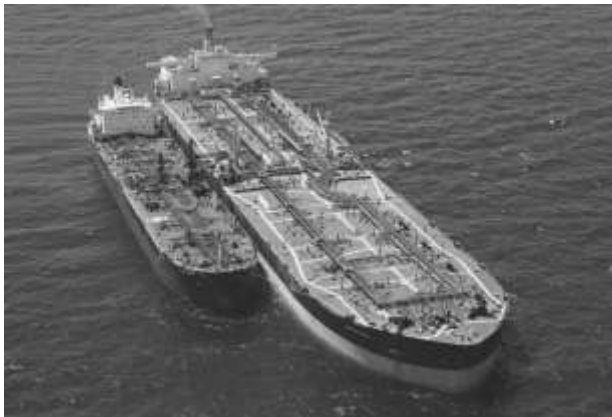
Fig 21 Ship to ship transfer operation
