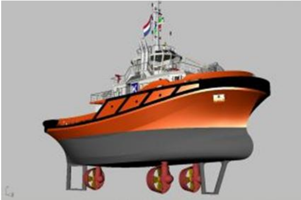
Fig. 8 Rotor tug with three rudder-propellers
