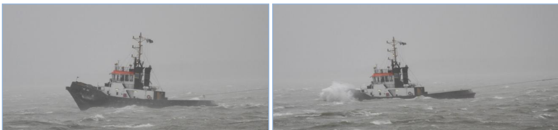
Fig. 27 Tug heaving and pitching on towline
