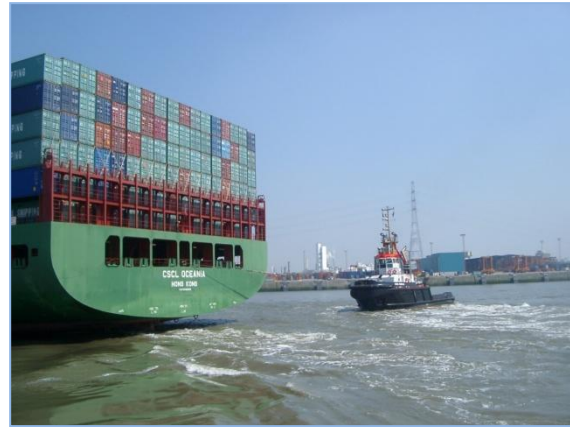
Fig. 12 ASD tug side steps to a position for assisting swinging
