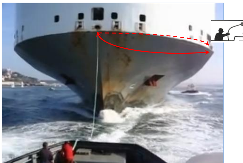
Fig. 19 Try to pass the heaving line to the ship's shoulder attached to a closed loop of line running back to the centre line chock inside the closed foc'sle
