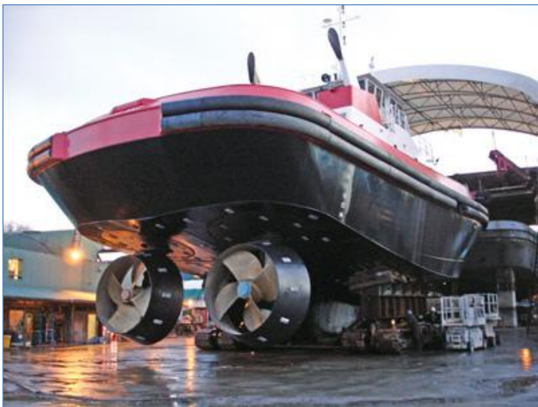
Fig. 5 Azimuth thrusters mounted at stern
