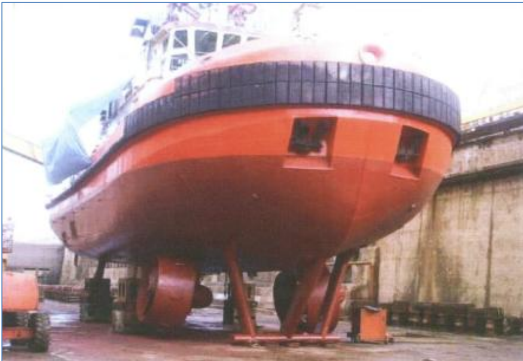
Fig. 6 Azimuth thrusters mounted at bow – water tractor
