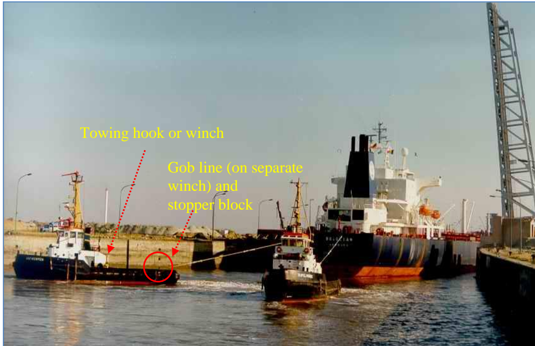
Fig. 3 Conventional tugs connected at the stern of the vessel being assisted.
