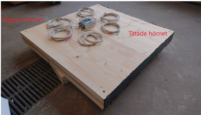
Preparation for measuring moisture content in a CLT element [1]
