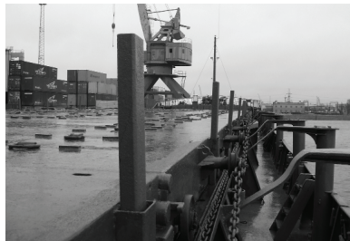
Figure 6.7. Example of uprights for bottom blocking
