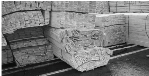
Figure 6.2. Example of poor rigidity
