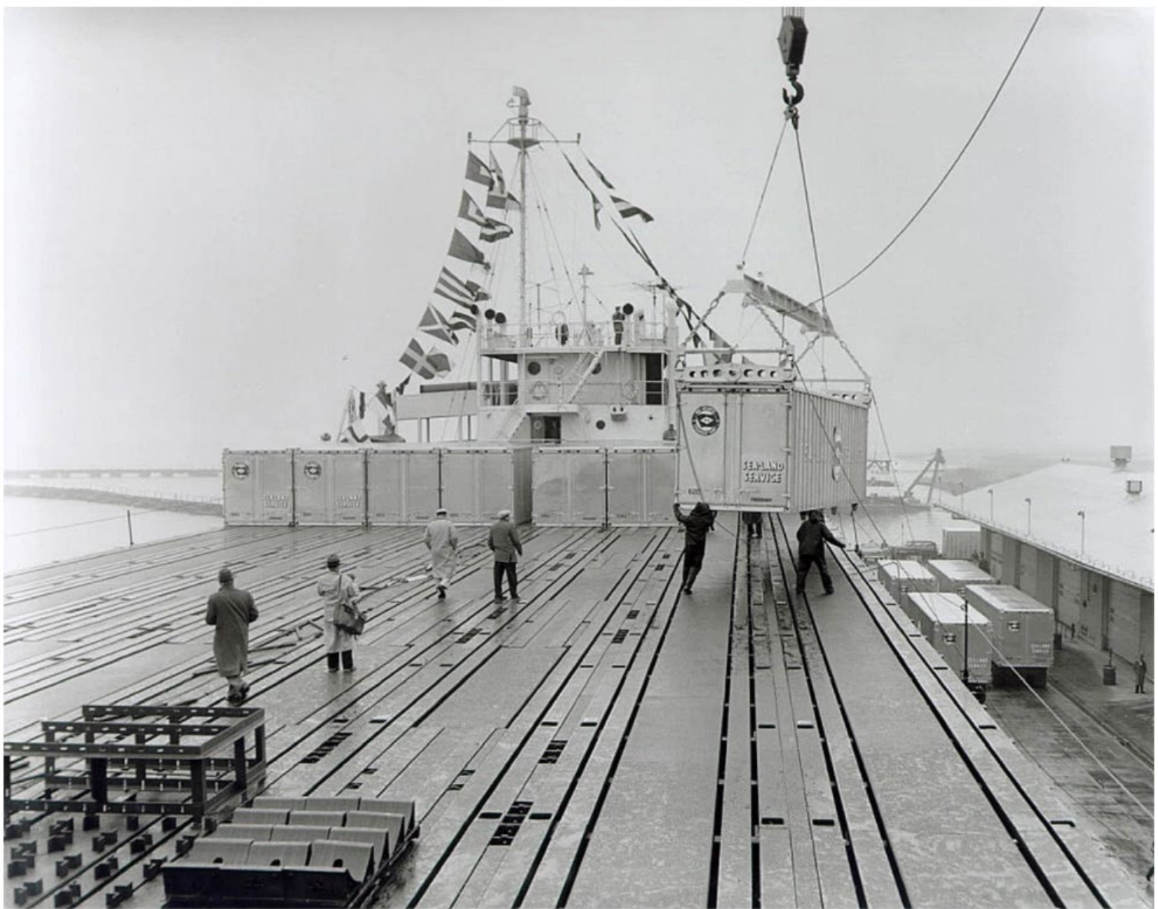
On 26th April 1956 a crane loaded the worlds first container ship with its cargo of ISO shipping containers in under eight hours. One container was loaded every seven minutes, a record at the time.
